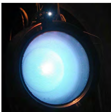
NASA's Evolutionary Xenon Thruster (NEXT) ion engine sets the world record for continuous operation.
