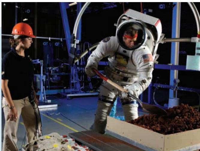
The Johnson Space Center's Life Support Systems and Environmental Control organization helps develop spacesuits for future human space flight. In one of the Center's laboratories, engineers test a suit's mobility during a basic task. (Credit: NASA)
