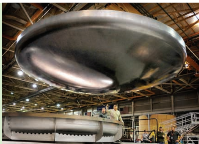
The Orion heat shield structure hovers above its layup mold during removal at the Lockheed Martin composite development facility. (Credit: Lockheed Martin)
